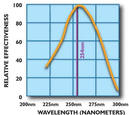
Approximately 95% of the ultraviolet energy emitted from **STER-L-RAY™** germicidal lamps is at the mercury resonance line of 254 nanometers, the region of germicidal effectiveness most destructive to bacteria, mold and virus.
